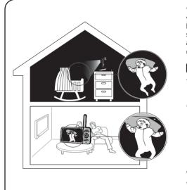
The baby unit has infrared LEDs that allow you to see your baby clearly at night or in a dark room. When the baby unit detects low light levels, the infrared LEDs are switched on automatically. The images from the baby unit are in black and white, and the appears on the parent unit screen.
